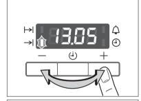
After approx. 5 seconds the display returns to showing the current time. The function indicator End time → lights up.
